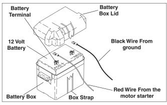
**STEP 8:** Place battery in battery box. Use a standard 12 volt battery.
