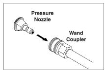
**STEP 3:** Pull spring-loaded collar of the wand coupler back to insert your choice of pressure nozzle.
