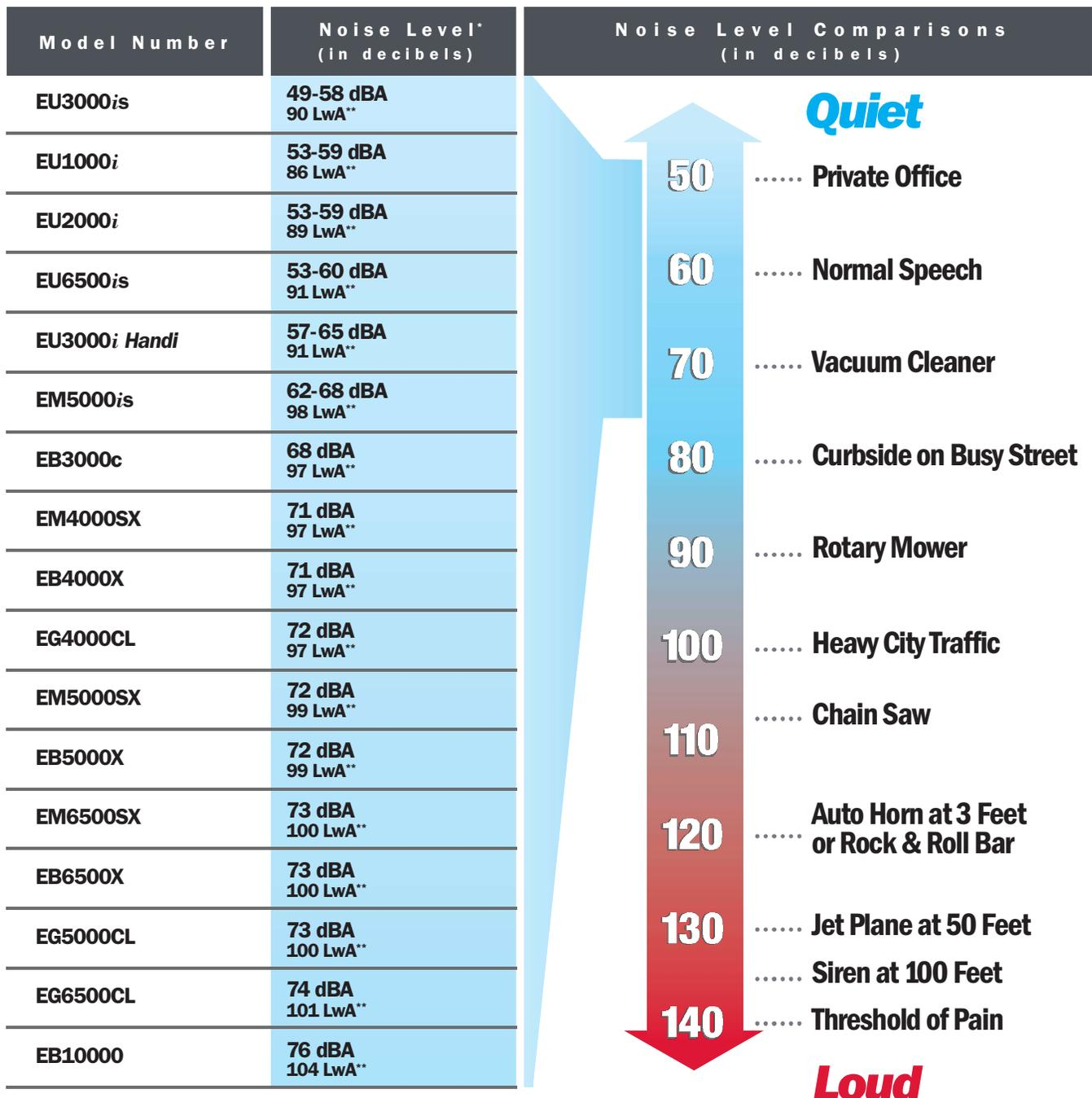
\* Noise levels at rated load to reflect maximum noise level possible, measured at 9 Feet (3 Meters) from the control panel side of the generator.
